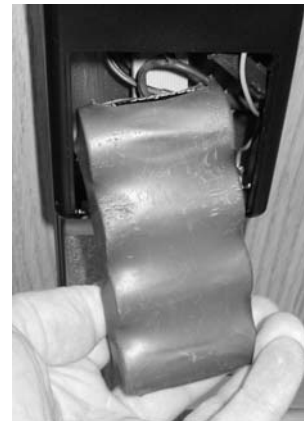
FIG. 18: INSERT BATTERY PACK INTO HOUSING
