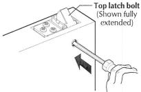
3. Check top latch bolt for deadlocking (latch bolt should not push in).
