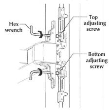
2. Open door and release top latch bolt as shown.
