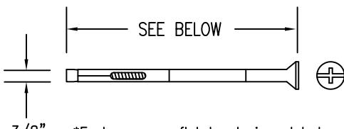
\*Fasteners are flat head zinc plated carbon steel dynabolt for masonry. Fastener lengths are shown below:
