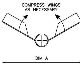
To install EO "butterfly" anchor, depress wings as necessary to suit depth (dim A). Hold one wing horizontal and position this wing under one of the backbends while placing tube over dimpled hole. Rotate anchor and snap remaining wing under opposite backbend.
