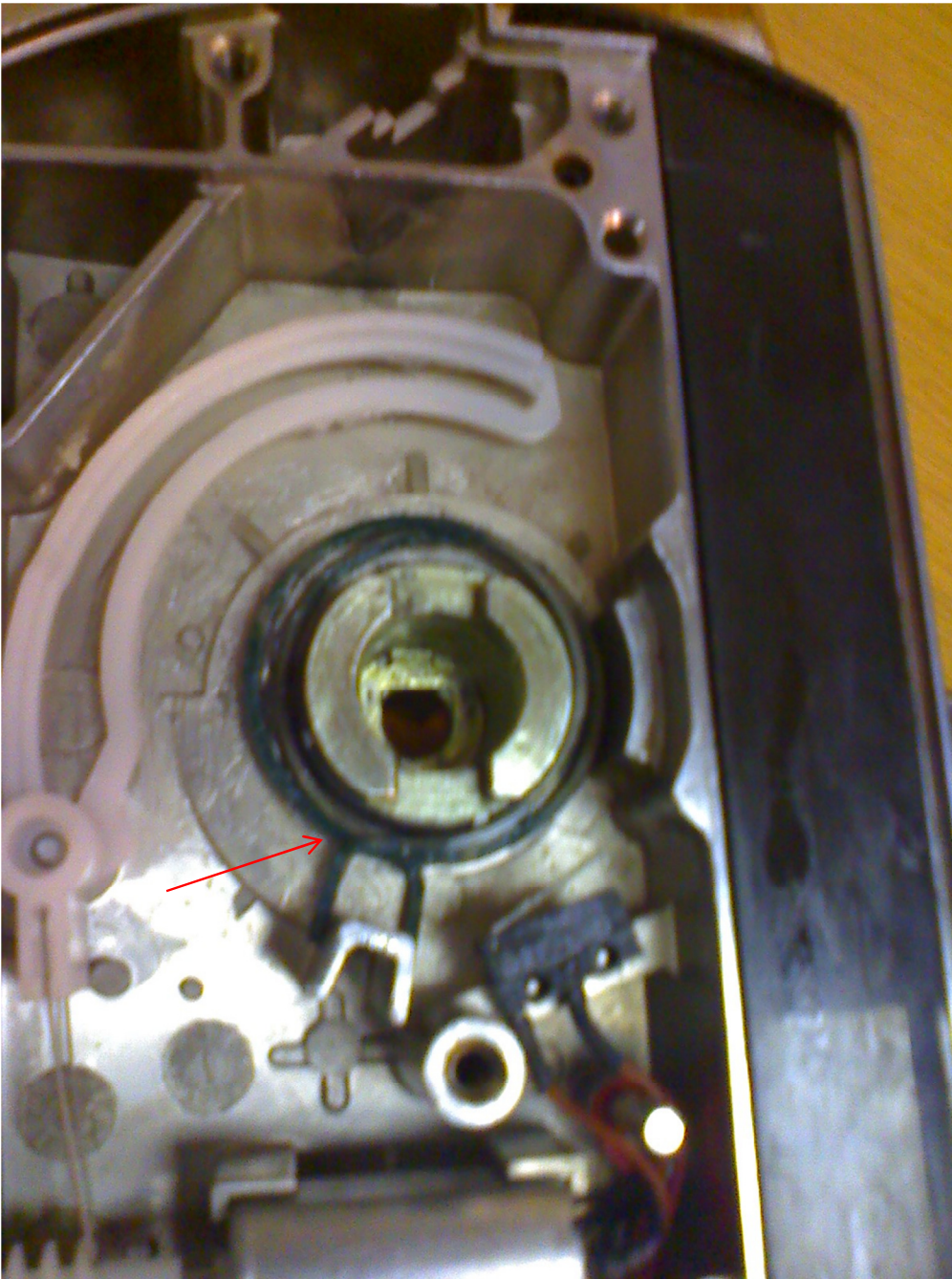
View of first spring to be install in front housing-Please note that the orientation in these pictures, the lock is upside down where the handle is away from you and the top of the lock is closest to you.
