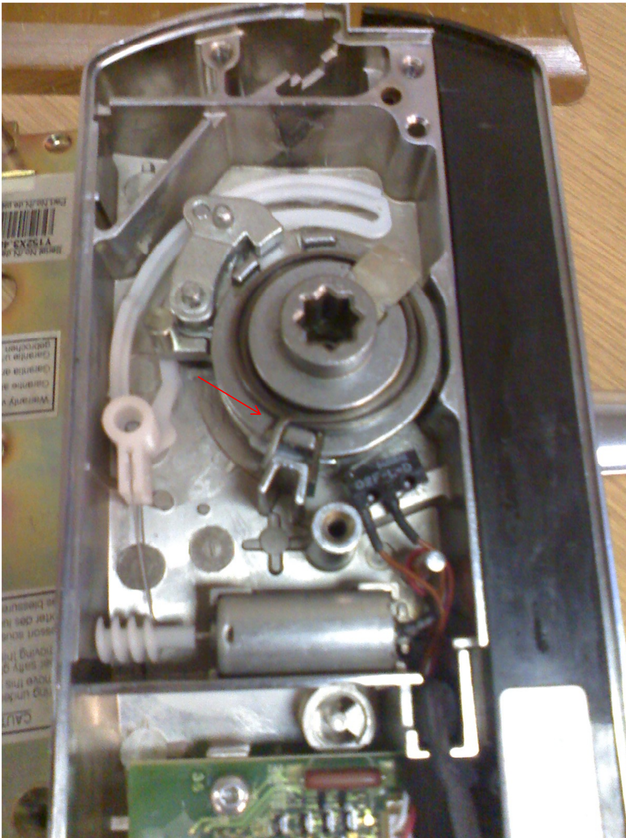
View of second lever spring installed in outer plate.
