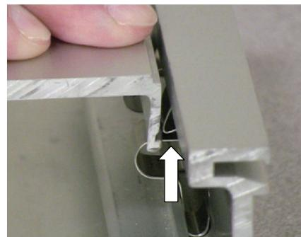
**10.** Insert a putty knife or small 1/8" straight screw driver (approximately 3/16" deep) between the exit device and filler plate directly above the top spring clip.
