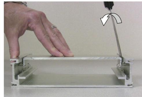
**12.** Repeat the above step to engage the filler plate with the other spring clip.
