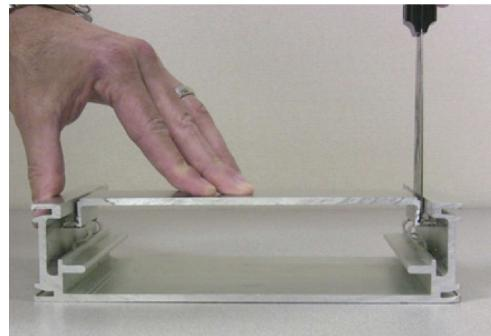
**11.** With the putty knife or small screw driver in place, **carefully pull down on the handle while pushing down lightly on the filler plate** to engage with a spring clip.
