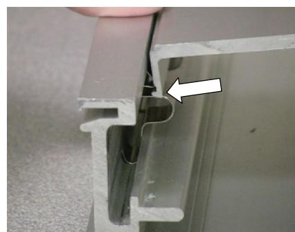
9. **Gently push the filler plate into a closed position**, engaging the top spring clips.
