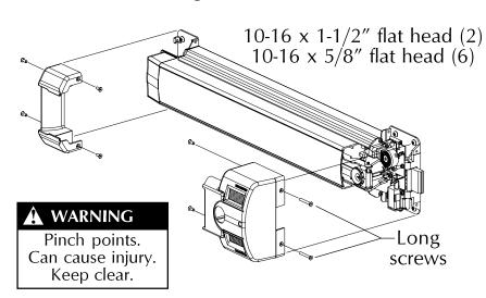
Close door and turn key 360 degrees each way. If dead bolt binds in single door strike, adjust strike as shown. Tighten screws. Prepare lockdown holes and install two lockdown screws as shown. Test device (see "Testing" on back of "Parts List").
