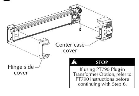
Mount center case to door. **Level** device before tightening screws.
